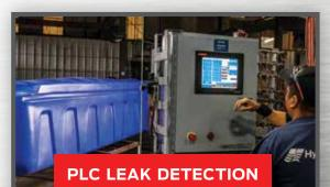
Pressure Decay Testing offers a unique and proprietary process which applies a predetermined PSI of air pressure to identify leaks.
